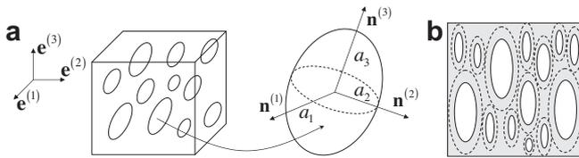
**Fig. 3.** Graphical representation of the microstructure. Part (a) shows the local orientation axes  $\mathbf{n}^{(i)}$  with  $i = 1, 2, 3$  of a representative ellipsoidal void with semi-axis  $a_1, a_2$  and  $a_3$ . Part (b) shows the a cross-section of the specimen where the “white” ellipsoids denote voids with ellipsoidal shape while the dashed ellipsoids refer to the distribution of their centers.
