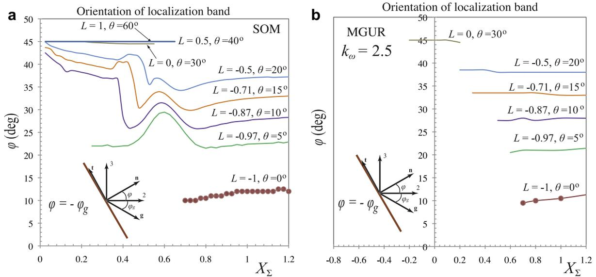
**Fig. 10.** Orientation of the localization band defined by the angle  $\varphi$  as predicted by (a) the SOM model and (b) the MGUR model with  $k_\omega = 2.5$ , as a function of the stress triaxiality  $X_\Sigma$  and the Lode parameter  $L$  (or  $\theta$ ). The strain hardening exponent is  $N = 0.1$  and the initial porosity  $f_0 = 1\%$ .
