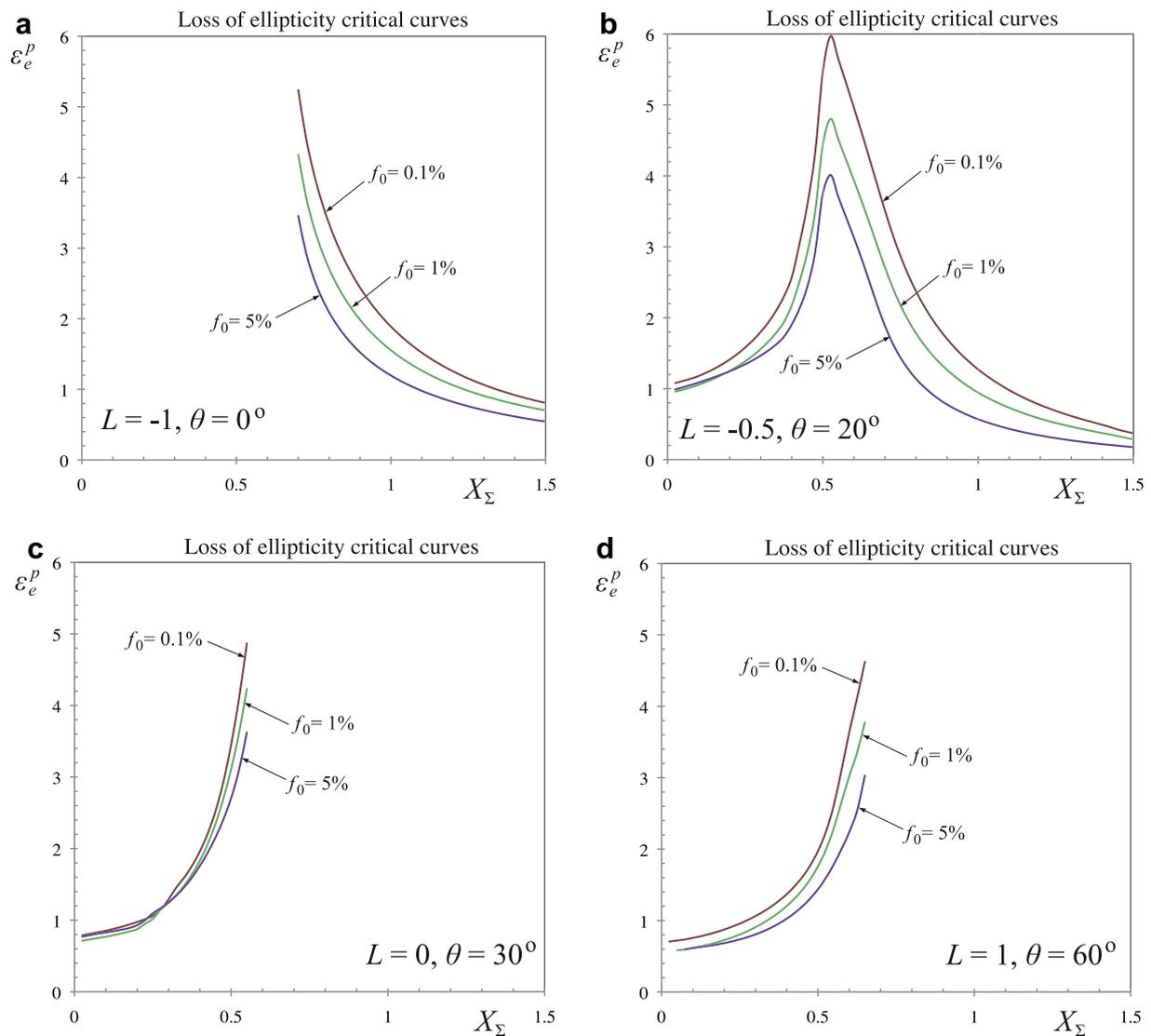
**Fig. 14.** SOM loss of ellipticity failure curves as a function of the stress triaxiality  $X_\Sigma$  and the initial porosity  $f_0 = 0.1, 15\%$  for various values of the Lode parameter: (a)  $L = 1$ , (b)  $L = -0.5$ , (c)  $L = 0$  and (d)  $L = 1$ . The strain hardening exponent is  $N = 0.1$ .
