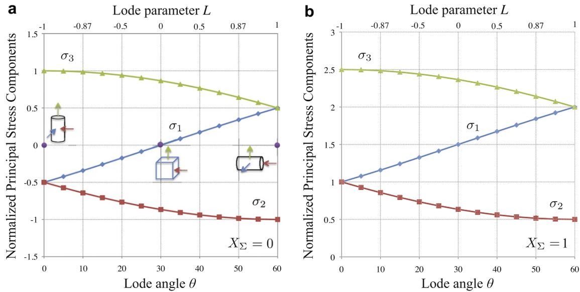
**Fig. 2.** Normalized principal stresses  $\frac{\sigma_i}{2\sigma_c} \{\sigma_1, \sigma_2, \sigma_3\}$ , as a function of the Lode angle  $\theta$  or equivalently the Lode parameter  $L$ . Parts (a) and (b) correspond to stress triaxialities  $X_\Sigma = 0$  and  $X_\Sigma = 1$ , respectively.
