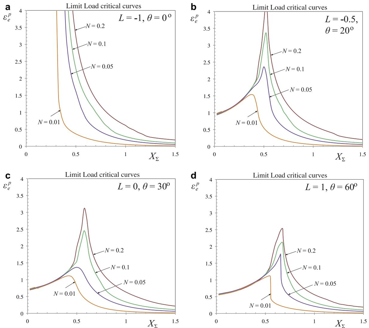
**Fig. 11.** SOM limit load failure curves as a function of the stress triaxiality  $X_\Sigma$  and the strain hardening exponent  $N = 0.01, 0.05, 0.1, 0.2$  for various values of the Lode parameter: (a)  $L = -1$ , (b)  $L = -0.5$ , (c)  $L = 0$  and (d)  $L = 1$ . The initial porosity  $f_0 = 1\%$ .
