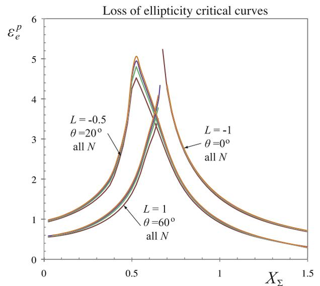
Fig. 12. SOM loss of ellipticity (LOE) failure curves as a function of the stress triaxiality  $X_\Sigma$  and the strain hardening exponent  $N = 0.01, 0.05, 0.1, 0.2$  for various values of the Lode parameter:  $L = -1, -0.5, 1$ . The initial porosity  $f_0 = 1\%$ .
