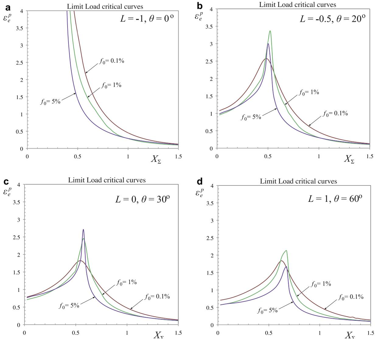
Fig. 13. SOM limit load failure curves as a function of the stress triaxiality  $X_\Sigma$  and the initial porosity  $f_0 = 0.1, 1, 5\%$  for various values of the Lode parameter: (a)  $L = -1$ , (b)  $L = -0.5$ , (c)  $L = 0$  and (d)  $L = 1$ . The strain hardening exponent is  $N = 0.1$ .
