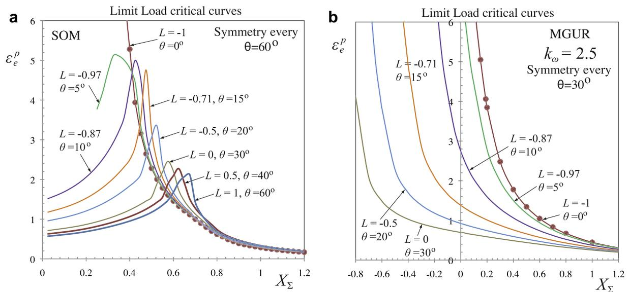
**Fig. 8.** Limit load failure curves as predicted by (a) the SOM model and (b) the MGUR model with  $k_\omega = 2.5$ , as a function of the stress triaxiality  $X_\Sigma$  and the Lode parameter  $L$  (or  $\theta$ ). The critical equivalent plastic strain  $\epsilon_e^p$  at the limit load where the hardening rate  $H = 0$  provides a “macroscopic” measure of the overall ductility of the material. The strain hardening exponent is  $N = 0.1$  and the initial porosity  $f_0 = 1\%$ .
